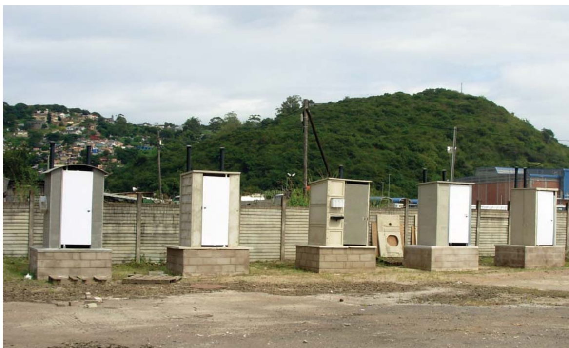
Demonstration of urine-diverting dry toilet prototypes, eThekweni, South Africa. Photo: Kim Andersson
