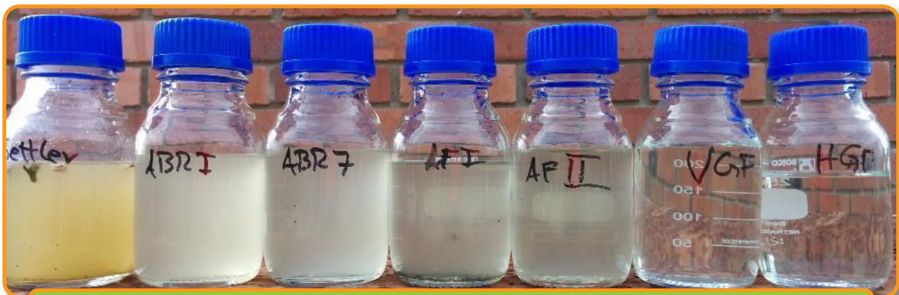
Photographs of samples taken through the Newlands Mashu DEWATS process. Abbreviations: ABR, anaerobic baffled reactor; AF, anaerobic filter; VGF, vertical flow wetland; HGF, horizontal flow wetland. Photos by Bjoern Pietruschka (2014).
