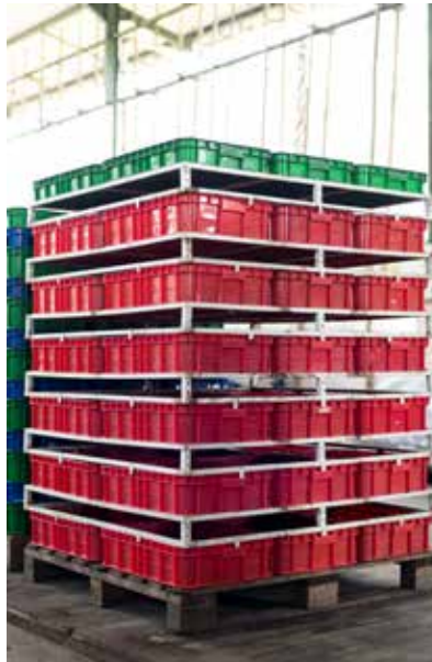
A stack of larveros. The metal frames allow ventilation and thus help water to evaporate from the waste ( T1-2 )
