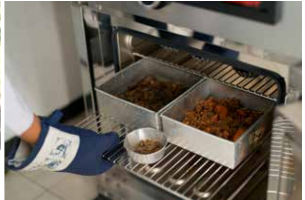
Samples for determination of dry matter content are put into the oven
