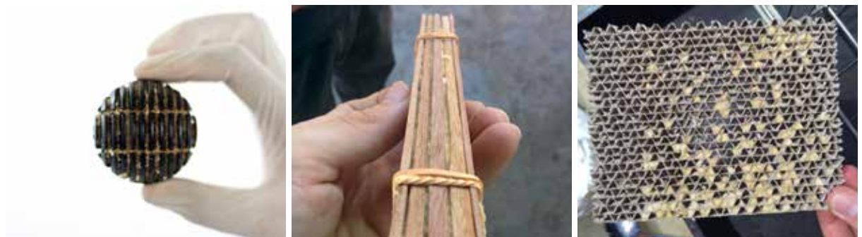
Figure 8: Different variants of eggies: "Bioballs", usually used as filter media in aquariums and ponds (left), stack of wooden sheets with small gap in between (middle), and cardboard honeycomb (right)
