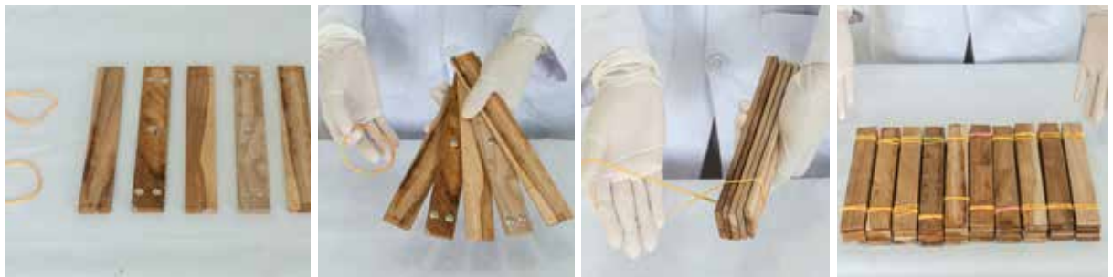
Wooden sheets with pushpins to create a gap, allowing space for egg packages. The eggies are held together with two rubber bands (R1-10)
