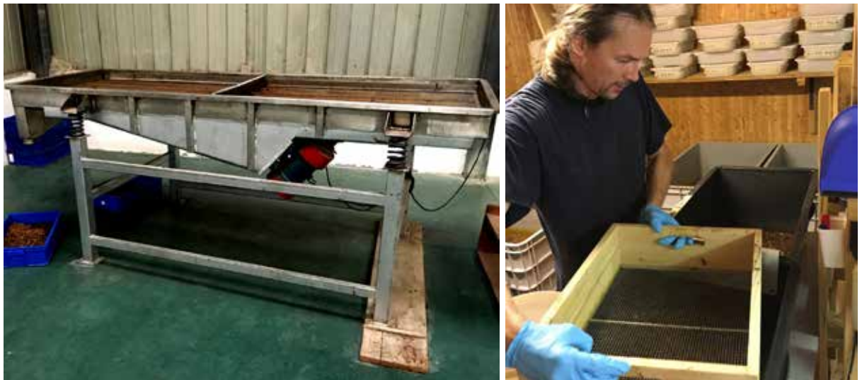
Figure 17: Shaking sieve (left) and manual sieve (right) to separate larvae from dry residue
