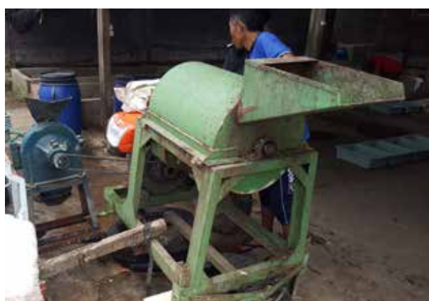
Figure 15: Hammer mill for waste pre-processing
